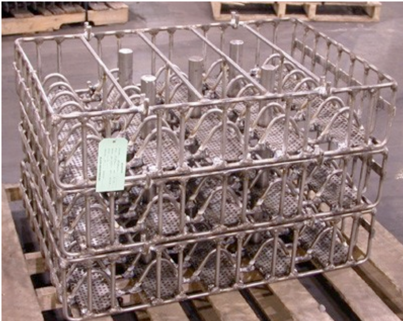
RA 602 CA alloy baskets designed for low pressure carburizing,
