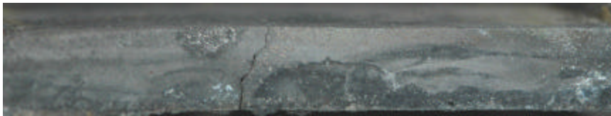
RA330 fracture surface, calcium LME. About 6X
