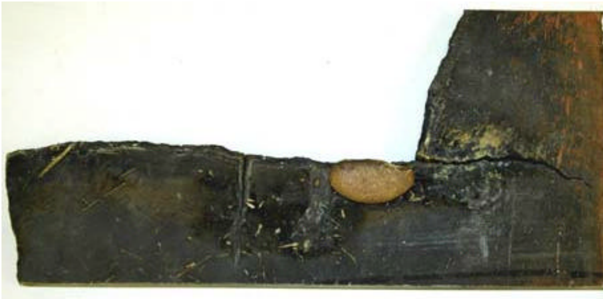
RA330 sintering muffle cracked by molten bronze
