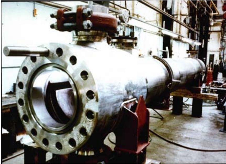
FIGURE 7 Heat exchanger supplied to Maersk Harald West project
