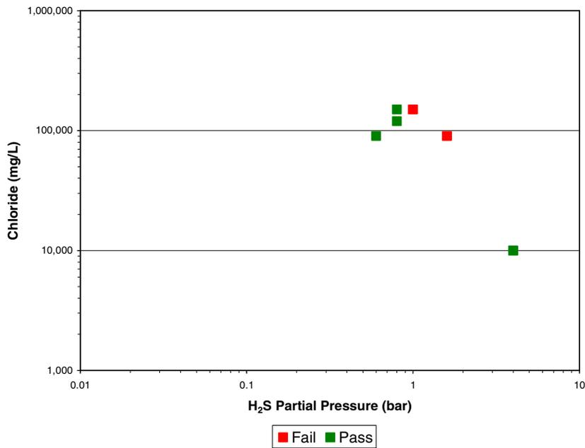
**FIGURE 5 Limits of use for Zeron 100 in sour brines**
