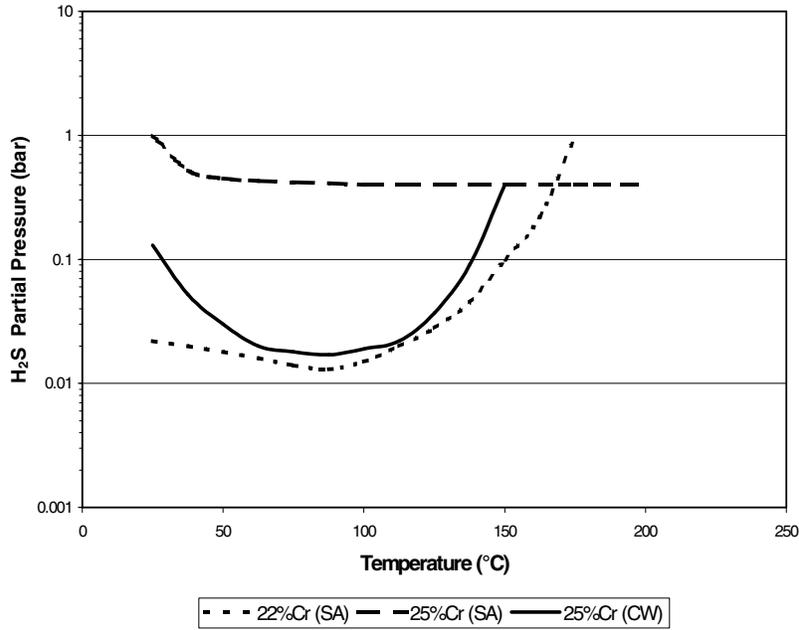
**FIGURE 2 Effect of temperature on the sulphide SCC resistance of heavily cold worked duplex stainless steels [Ref 5]**
