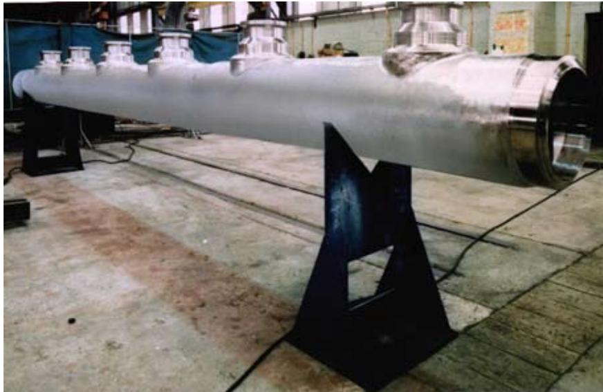
FIGURE 9 Section of Marathon East Brae manifold during Fabrication
