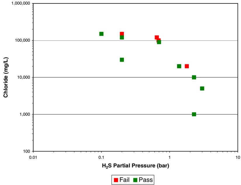
**FIGURE 4 Effect of chloride on sulphide
