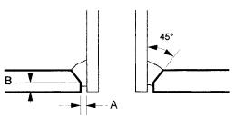
Gap A = 1/16 to 1/8 inch (1.6 to 3mm) Land B = 1/16 to 1/8 inch (1.6 to 3mm)
