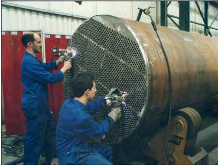
FIGURE 10. Condenser in Zeron 100 for a VCM plant
