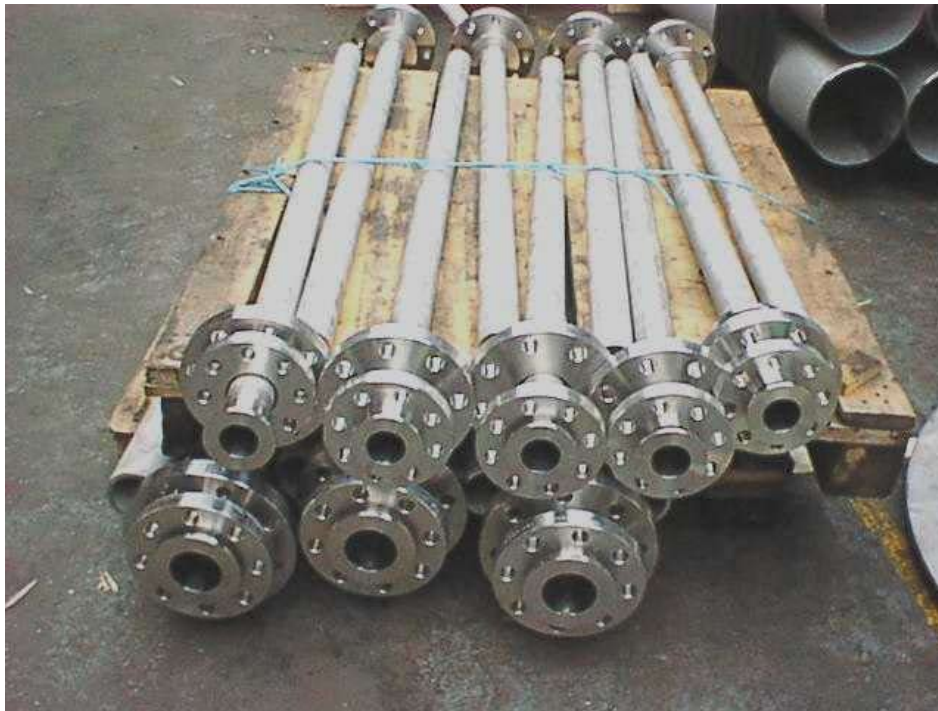
FIGURE 10 Oxygen sparge pipes for main autoclave at Lihir gold mine, PNG
