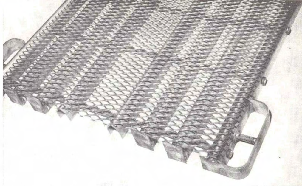
Typical base tray of "barn-roof" design shows articulated fabrication with tie rods and spacer tubing. This one was made of 330 alloy steel
