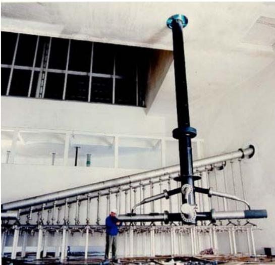
**Figure 2: N08367 Alloy Rotary Sparger**
