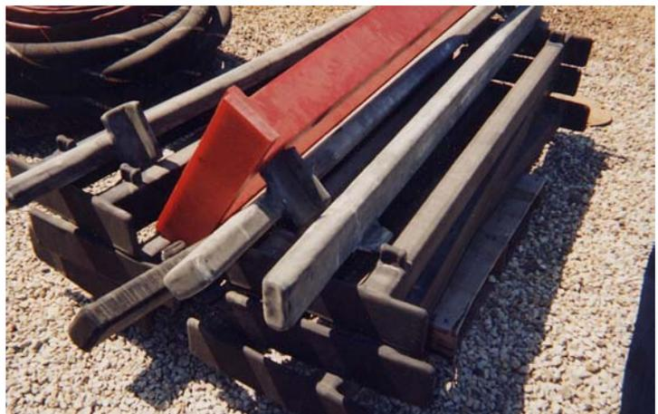
**Rubber Coated Carbon Steel Beams**
