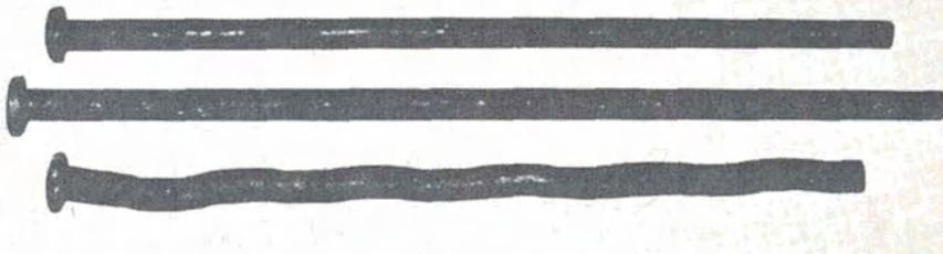
Fig. 6 — These three pins operated in the same furnace for three years at temperatures ranging between 1,550 and 1,750 F. The distorted pin (bottom) is of coarse-grained 32 Ni, 21 Cr alloy, while the other two are of RA 333-SA, a more highly alloyed material.
