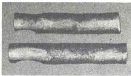
Fig. 5 — Though different in grain size, the pins of Fig. 4 exhibited practically the same degree of crankshafting in service. The lower pin has the coarser grains.
