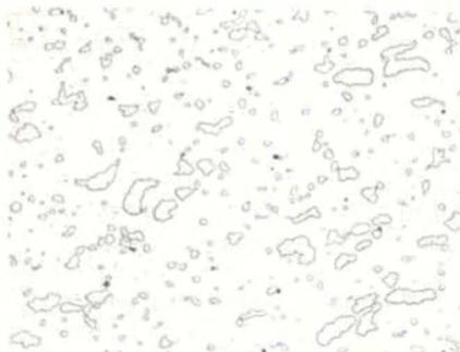
Fig. 1 — This belt pin, of RA 330-HC, became severely distorted during a year's service in a stress relieving operation at about 1,650 F under a loading of approximately 16 lb per sq ft. Micro (250X) shows massive carbides; compare with Fig. 2.
