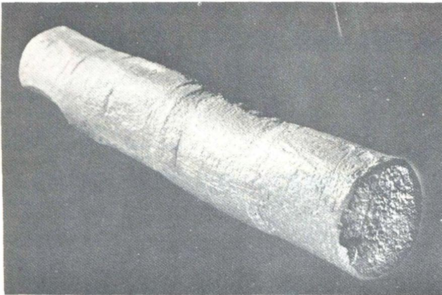
Fig. 3—This belt pin apparently failed because of mechanical fatigue. Note crack midway along the bar. This pin was cleaned by pickling.
