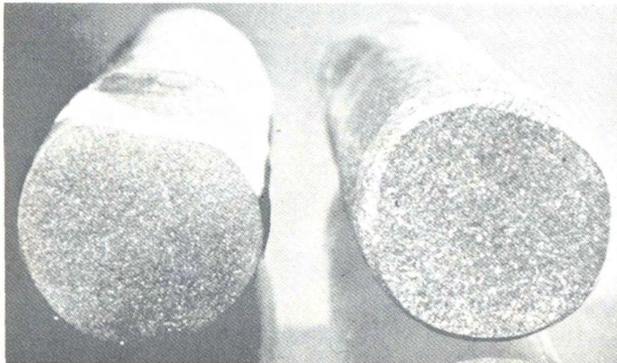
Fig. 4—These two pins have different grain sizes. The coarse-grained stock (right) has a slightly lower nickel content, 32%. Etchant, 50% HCl in water (160 F); approx. 2X.
