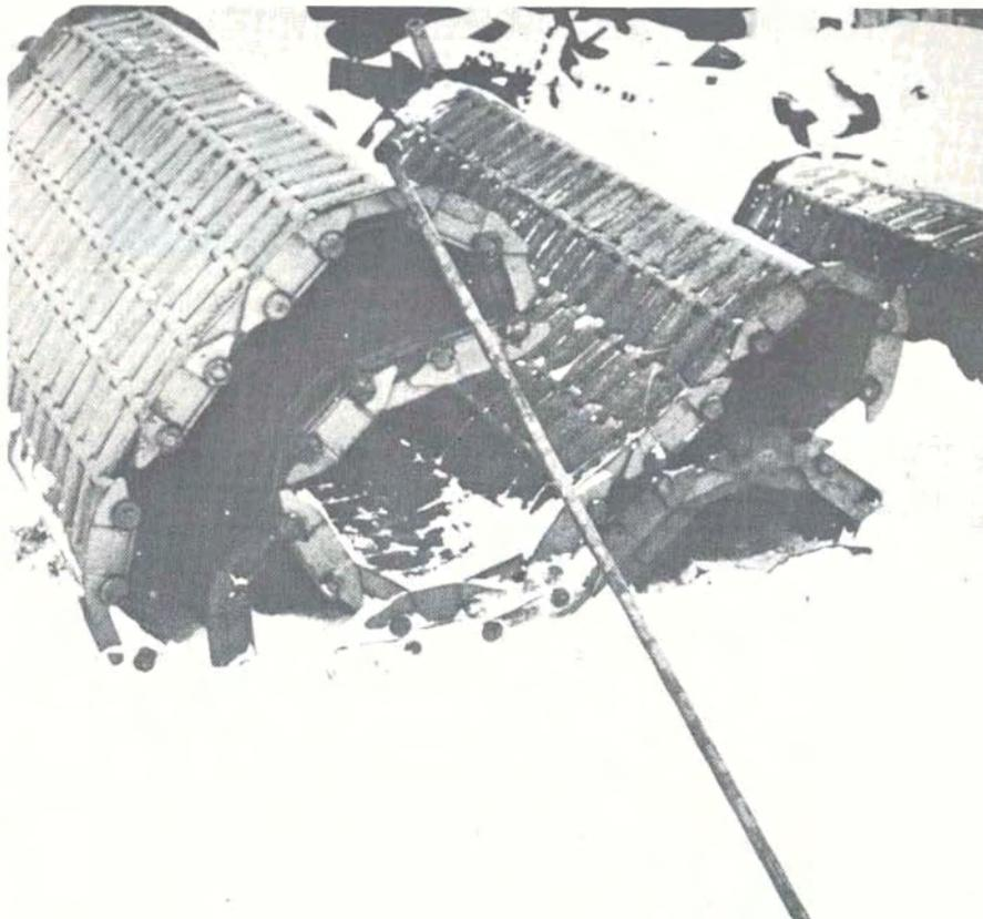
Belt pins of RA 333-SA are still straight even though the belt had to be scrapped. It served more than five years in a furnace operated between 1,550 and 1,650 F.
