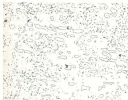
Fig. 2 — Though representing the same heat of material in the same application as the pin of Fig. 1, this pin was only slightly deformed ("crankshafted") after the same year of service. The cause is attributed to a different annealing cycle — unlike the pin of Fig. 1, this pin had fine, well dispersed carbides, shown at 250X in the micro.
