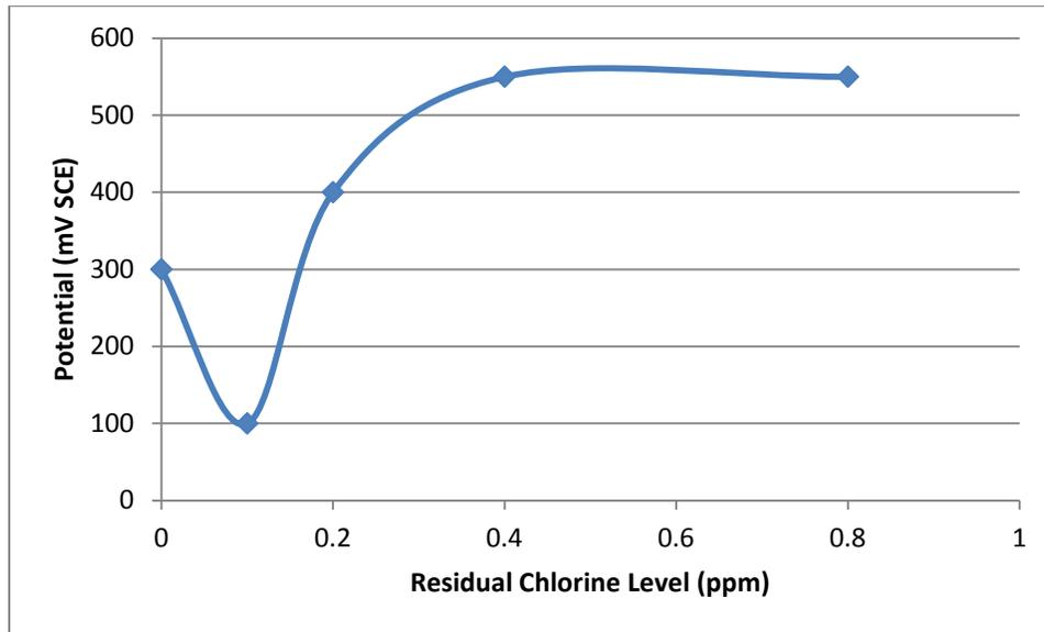
Figure 2: the Relationship between the Potential of SDSS in Seawater and Residual Chlorine level
