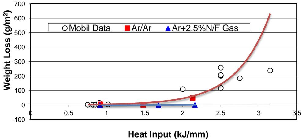
Figure 10: The Variation of Weight Loss Results of Welded Joints made with a Range of Heat Inputs and Welding Gas Combinations when Exposed to Ferric Chloride Solution at 40°C for 24 Hours
