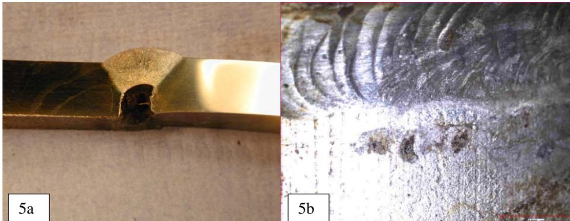
Figure 5: a) Weld Root Run Corrosion and b) LTHAZ Corrosion Attack
