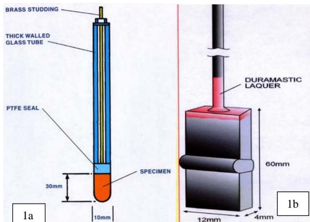
Figure 1: a) Schematic Diagram of the Assembly Used to Measure RCCT (Silicone O Ring Seal Omitted for Clarity) and b) Schematic Diagram of Welded Sample Used to Measure CPT.
