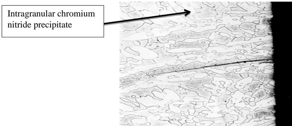
Figure 12: the Microstructure in the Region of Cracking of Failed Hub connector (etched electrolytically in Oxalic Acid and Potassium Hydroxide)
