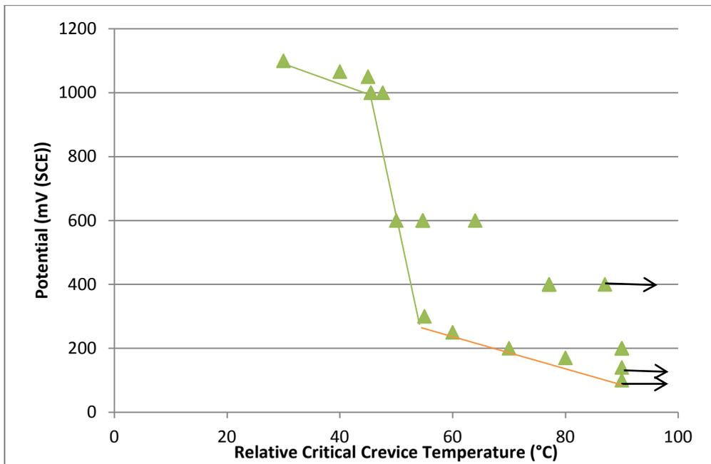
Figure 3: the Effect of Potential on RCCT for Z100 Parent Material in Seawater Solution
