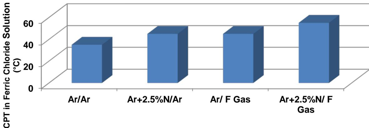
Figure 8: the Effect of Shielding Gas/ Backing Gas Combinations on CPT of Welds in Ferric Chloride Solution
