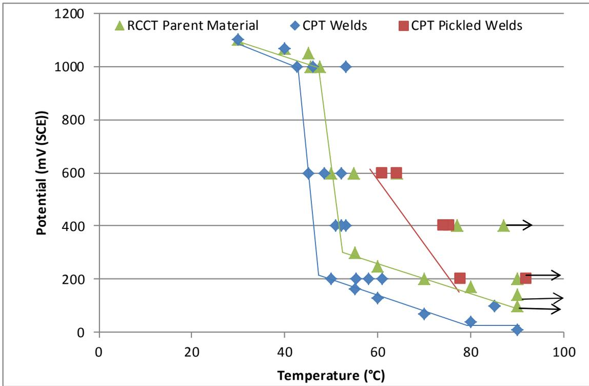
Figure 11: Variation of RCCT of Parent Material and CPT of “As Deposited” and Acid Pickled Welds in Seawater Solution
