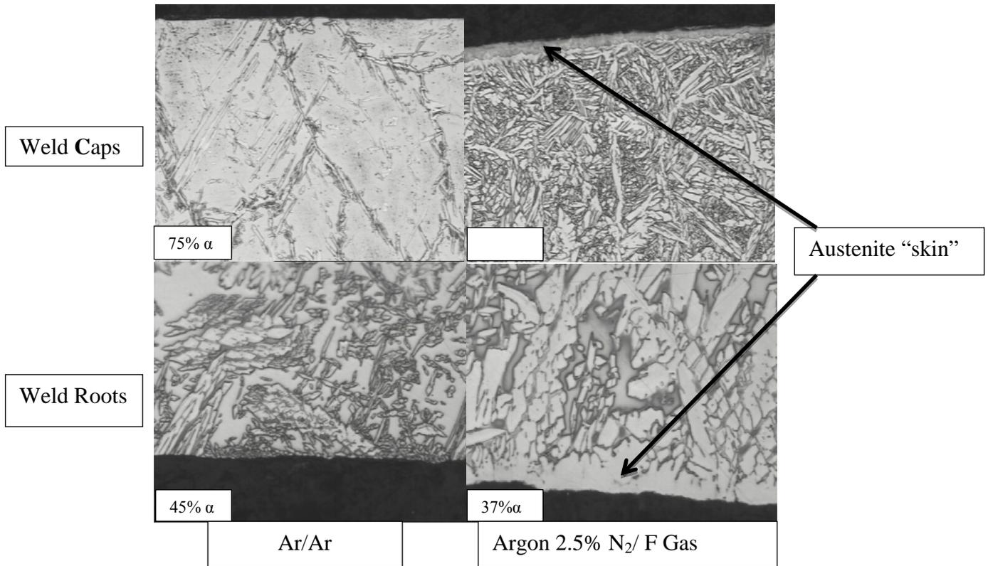
Figure 9: The Microstructures of Welds Deposited Using Pure Argon for Both Shielding (Ar/Ar) and Backing Gas and Argon +2.5% N<sub>2</sub> Shielding and F Gas backing gasses (samples etched electrolytically in Oxalic Acid and Potassium Hydroxide)
