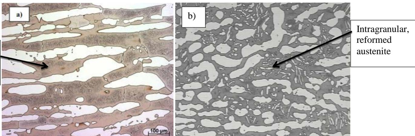
Figure 14: The Microstructure of a) UNS S 32760 Forging with a High Level of Intragranular Chromium Nitride Precipitate<sup>31</sup> and b) a Z100 Modified Forging with Intragranular Reformed Austenite (etched electrolytically in Oxalic Acid and Potassium Hydroxide)
