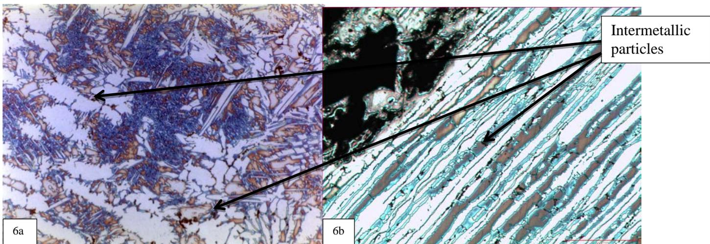
Figure 6: a) Weld Metal and b) LTHAZ Intermetallic Particles (samples etched electrolytically in Oxalic Acid and Potassium Hydroxide)
