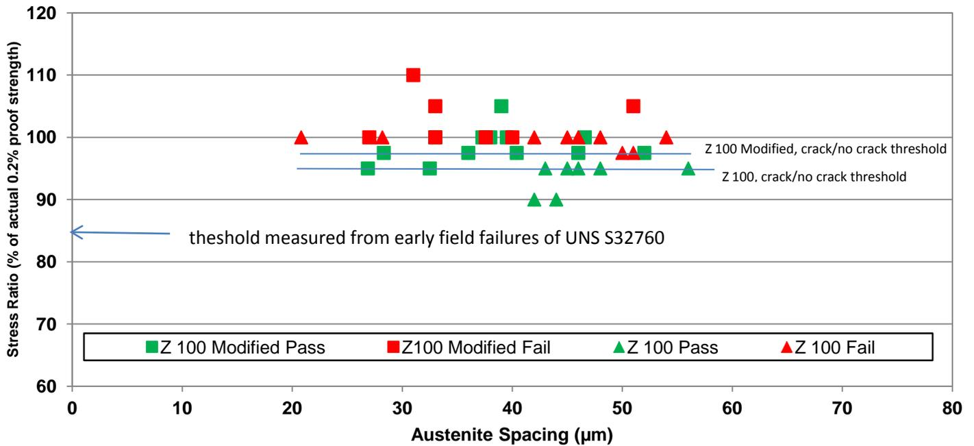
Figure 13: Summary of Constant Load Tests of Z100 and Z100 modified Samples from Forged 10k Weld Neck Flanges Exposed to Seawater and Polarized to -1.04V (SCE)
