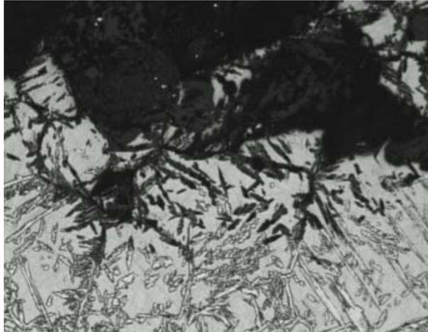
Figure 7: Preferential Attack of Austenite in the Weld Root (samples etched electrolytically in Oxalic Acid and Potassium Hydroxide)
