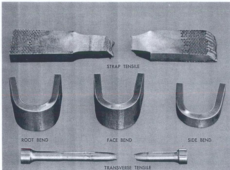
Fig. 6 Weldments of RA 330 welded with RA 330-04-15 illustrating both strength of the weld deposit metal and ductility of the overall weldment.
