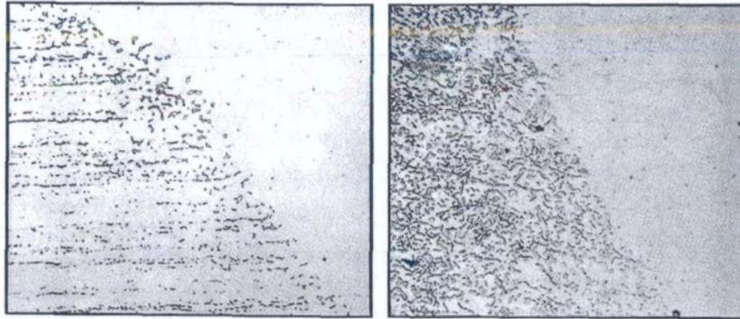
Fig. 9 Fusion zone between 309 parent metal (left hand side of 9A) and RA 330-04 bare wire. The deposit metal is fully austenitic while the ferrite content of the base metal as determined by a Magne-Gage was one percent in the as-welded condition. After sigmatizing (9B) about 20% sigma can be noted in the base metal (left hand side of 9B) while the weld deposit metal has remained fully austenitic. Magnification 235X (Reduced 10%). Etchant, Vilella's.
