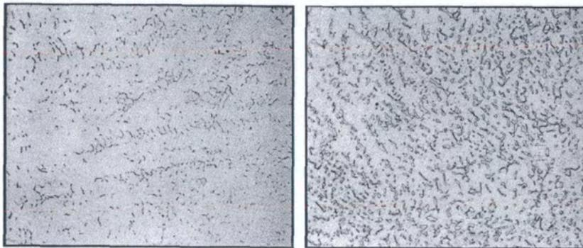
Fig. 10 Type 309-16 weld deposit metal in the as-welded condition and in the sigmatized condition (10A and 10B, respectively). Magnification 235X (Reduced 10%). Etchant, Vilella's.
