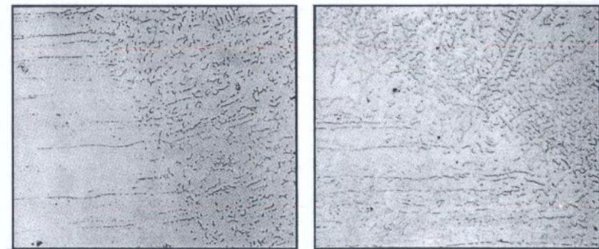
Fig. 8 Fusion zone between 309 parent metal and 309-16 weld deposit metal as welded (8A) and after sigmatizing for 1000 hours at 1400°F (8B). Magne-Gage ferrite content determination of weld deposit metal 7%. Parent metal on left hand side of micrographs. Magnification 235X, Etchant, Vilella's (Reduced 10%).
