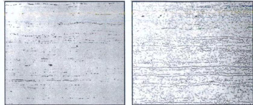
Fig. 7 Type 309 parent metal in the as-received condition (7A) showing about 1.5% ferrite present and after sigmatizing (7B) at 1400°F for 1000 hours showing about 20% sigma present. Magnification 235X, Etchant, Vilella's (Reduced 10%).
