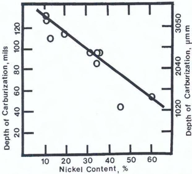
Figure 7— Effect of Nickel on Carburization
