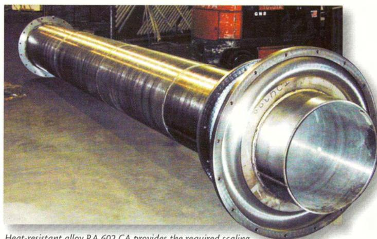
Heat-resistant alloy RA 602 CA provides the required scaling resistance and creep strength for calciner used to process metal oxides.
