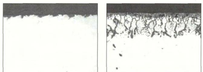
**Fig 3** Surfaces of RA 602 CA (left) and Alloy 601 (right) after 3,150 hours exposure at 2100°F.
