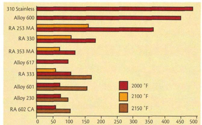
**Fig 1** Oxidation rates for selected heat-resistant alloys at temperatures between 2000 and 2150 °F. Samples were cycled weekly to room temperature over a test period of 1,500 to 3,400 hours. Source: Ref 2, 3.
