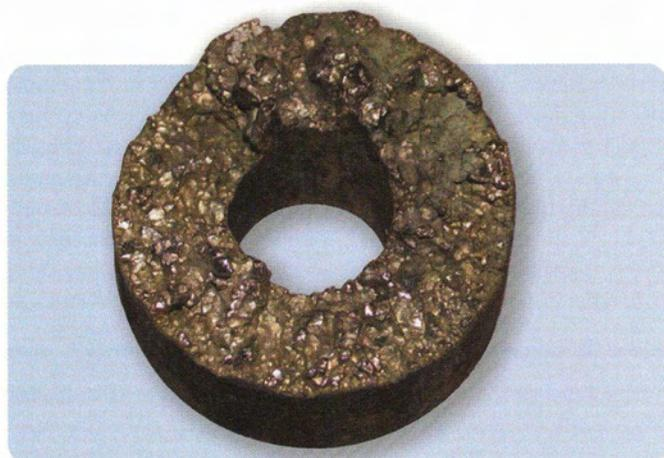
Fig 4 Fracture surface of a failed Alloy 600 thermocouple sheath taken from a molten-salt pot operating at temperatures in excess of 2100°F. Extensive grain growth has occurred due to overheating.
