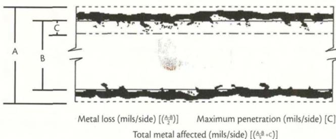
**Fig 2** High-temperature oxidation metrics
