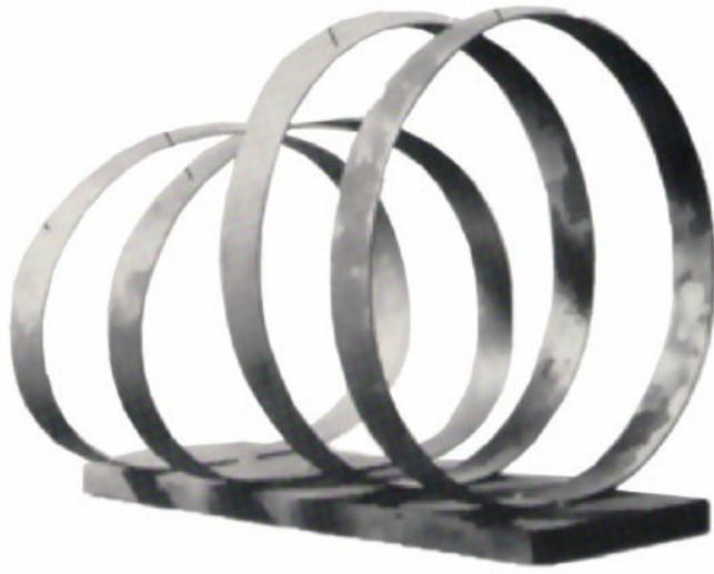
Fig. 3. Photograph illustrating creep. The least creep is observed in alloy RA253MA and worst in 321.
