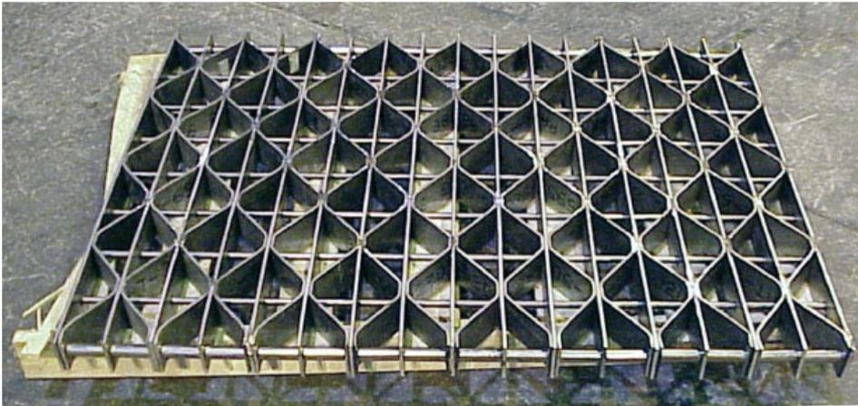
Fig. 4. Serpentine grid. Note that the only welds are between the nut and the threaded rods holding the entire assembly together and allowing freedom of movement during expansion and contraction.
