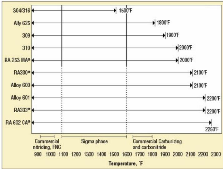
Fig. 1. Oxidation limits of some heat-resistant alloys. Note that for alloy 600, different sources limit this alloy to 2000°F.
