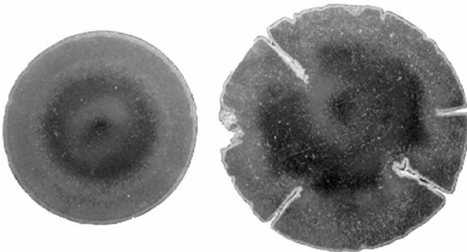
Fig. 5. (left) 0.5-inch (12.7-mm) diameter, RA330 basket top frame. (right) 0.625-inch (15.9-mm) diameter, RA330 from same heat treat basket
