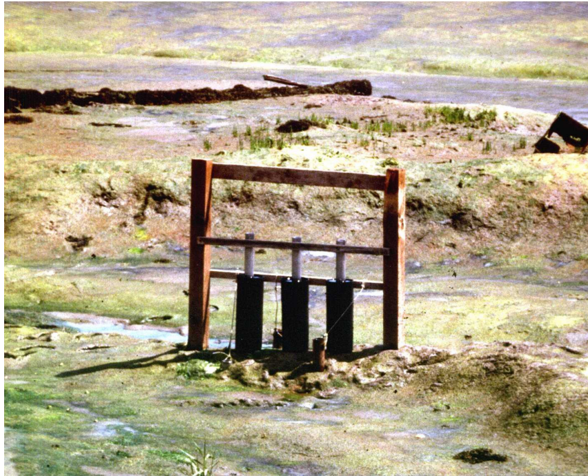
Figure 8 The appearance of the MIC test frame at low tide.
