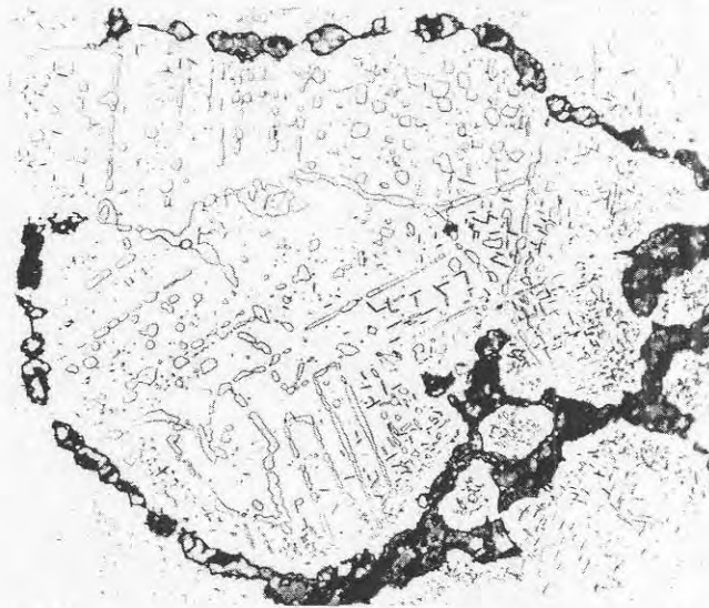
Fig. 4 Microstructure of sample shown in Fig. 3 evidences semi-continuous network of chromium carbides on grain and twin boundaries as well as being distributed in the matrix. Etchant: Mixed acids. Magnification 500X (reduced 5%).
