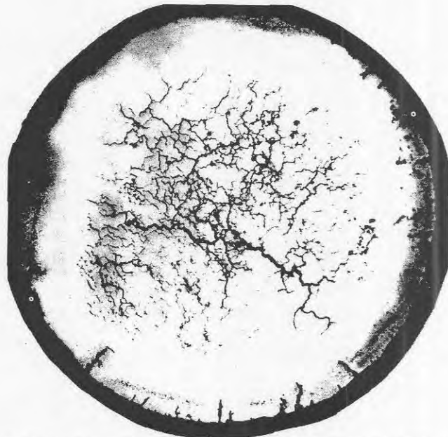
Fig. 3 Internal thermal fatigue cracks in cross section of \frac{1}{2} " diameter RA-330 bar frame basket.
